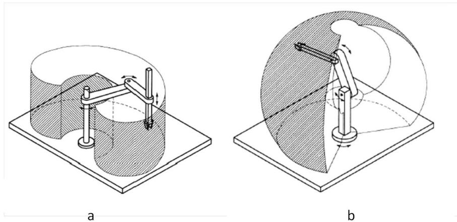
Figure 1. The basic structures 3R (a-scale structure ; b-anthropomorphic structure)
