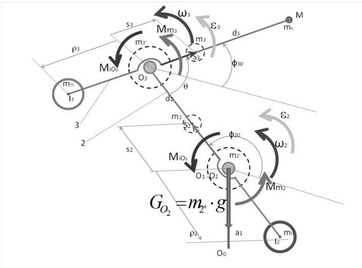
Figure 7. Dynamics of the kinematic chain plan balanced
