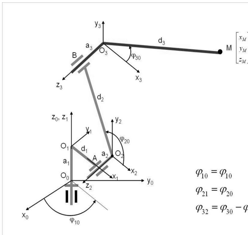
Figure 3. Layout geometro-cinematic a modern structures 3R (anthropomorphic)
