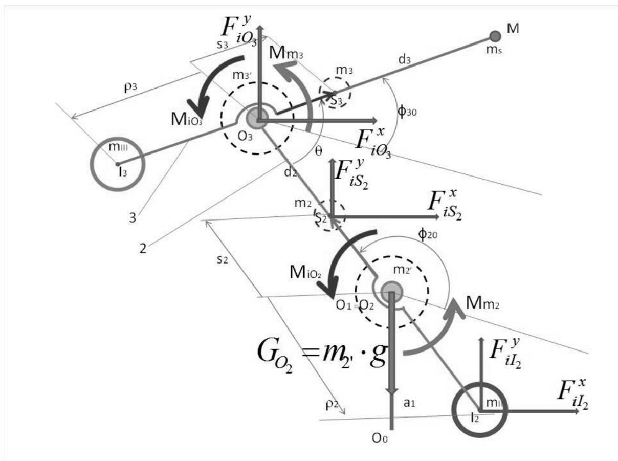
Figure 6. Forces of the kinematic chain plan balanced
