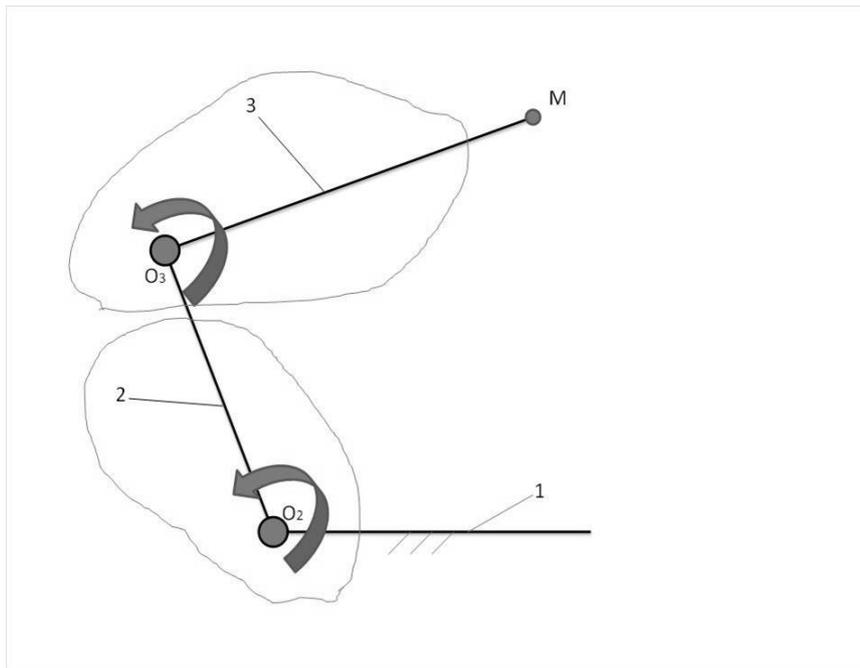
Figure 4. Structural schematic kinematic chain plan 2-3 linked to item 1 considered fixed
