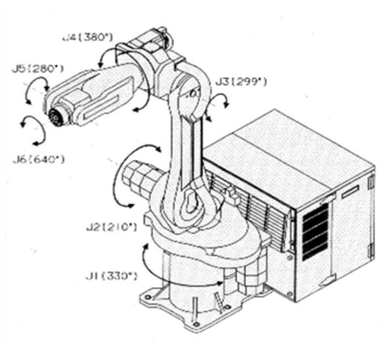
Figure 2. Structure 6R (anthropomorphic structure)
