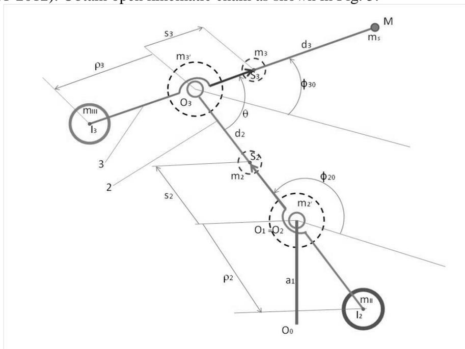
Figure 5. Static total balance of kinematic chain plan
