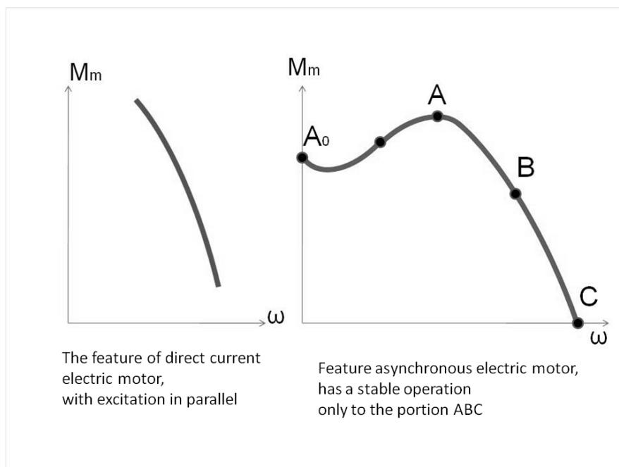
Figure 8. Electric motors feature
