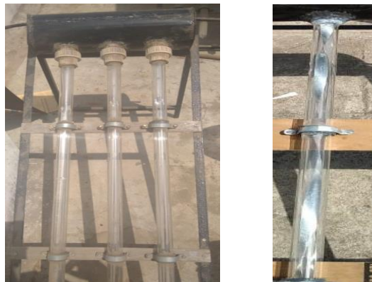
Fig. 1 - Experimental Set Up; Fig. 2 - Evacuated Tube with Twisted Tape
