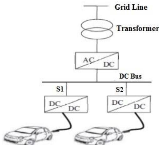
The schematic diagram shown in Fig. 6 can be used to illustrate how a charging station operates and how electricity flows through it. A battery adapter (DC/DC converter) connects the electric vehicle to the charging station's DC bus. Constant Current-Constant Voltage (CC-CV) charging is the charging system used to charge the battery of an electric vehicle.
