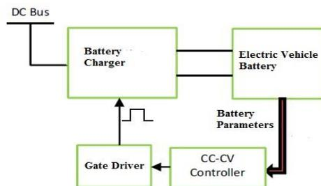
Fig. 8 - Charging Flow Map for CC-CV
