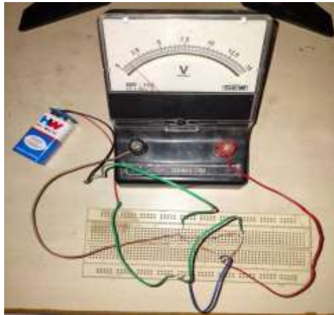
Fig. 2a- Wheatstone Bridge with Solid State Resistor. Voltage Deflection Measured is 1 Volt
