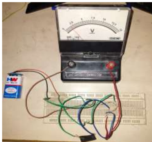
Fig. 2b- Wheatstone Bridge Circuit with Graphene PVDF Film. Voltage Deflection Measured is 2 Volts
