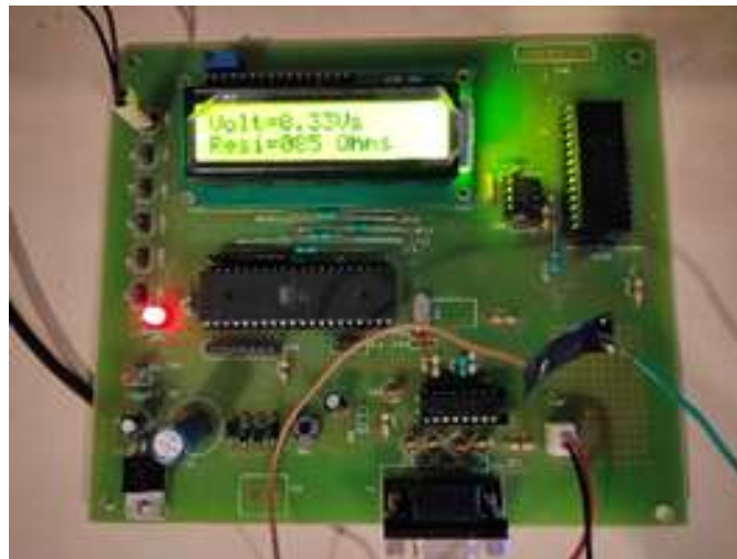
Fig. 1- Embedded Hardware Showing Voltage and Resistance Reading when Pressure is Applied to Graphene PVDF Film
