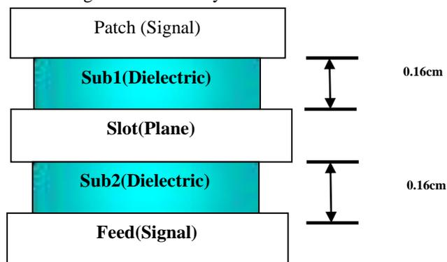
The radiating patch separated from the lower layer by a ground plane. The bandwidth is determined by the amount of coupled power, and the largest bandwidth can be obtained by minimising spurious feed radiation by making direct contact between the feed and the patch. In the proposed framework, two dielectric layers of varying thicknesses are distinguished by a ground plane with a slot that ties the RF power to the patch.
