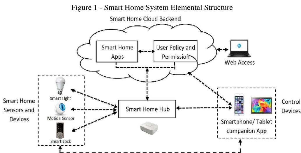
Smart Home Systems, shown in Figure 1, are usually hardware modules composed of cameras, smart objects, gateways, and sensors. The separate one component categories are:
