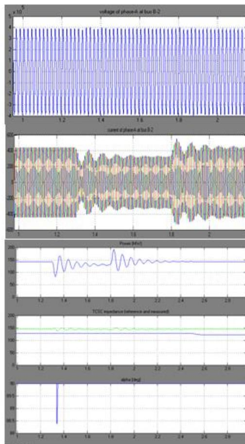
**Map: 4.** Variations of Generators Potential differences in Amplitude are:(I) phase – A voltage at Bus bar B - 2, (II) phase – A current at Bus bar B – 2, (III) TCSC power flow, (IV) TCSC impedance and (V) TCSC angle.
