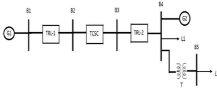
**Fig:1.**Flow diagram of the proposed test system.
