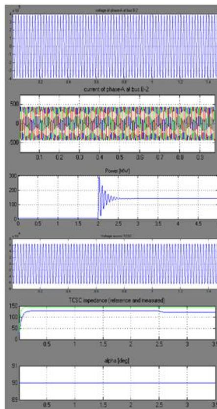
**Map: 6.** Turning the load to the off state (I) phase – A voltage at Bus bar B - 2, (II) phase – A current at Bus bar B – 2, (III) TCSC potential difference, (IV)TCSC power flow, (V) TCSC impedance and (VI) TCSC angle.
