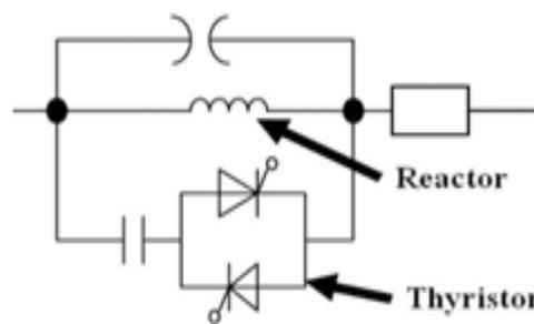
**Fig:2.** Schematic figure of the TCSC
