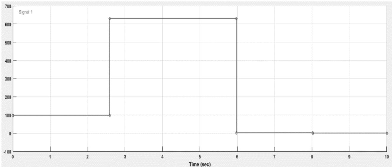
The source for solar panel is sun and since the source does not have constant value it is chosen to be in pulse with three different signals, low radiation, high radiation and zero radiation. The converter will take care of delivering constant supply throughout the system.
