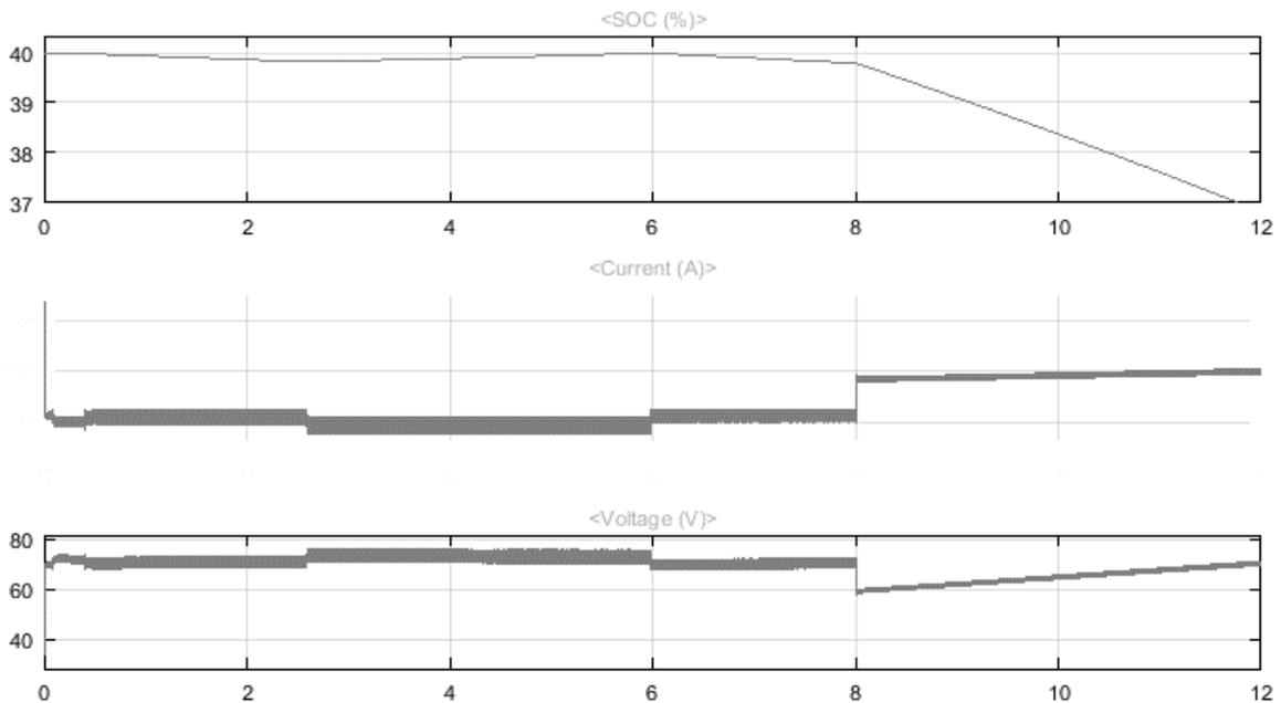
State of charge is associated with battery tells how much power can it deliver in ampere hours (Ah). At a particular time when battery loses its energy the voltage drops and current raises. In this situation, the bidirectional port is used to recharge the battery. Simultaneously, other source comes in.
