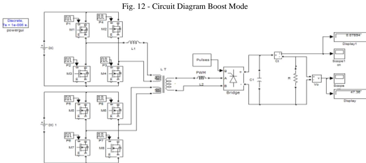
Fig. 12 - Circuit Diagram Boost Mode
