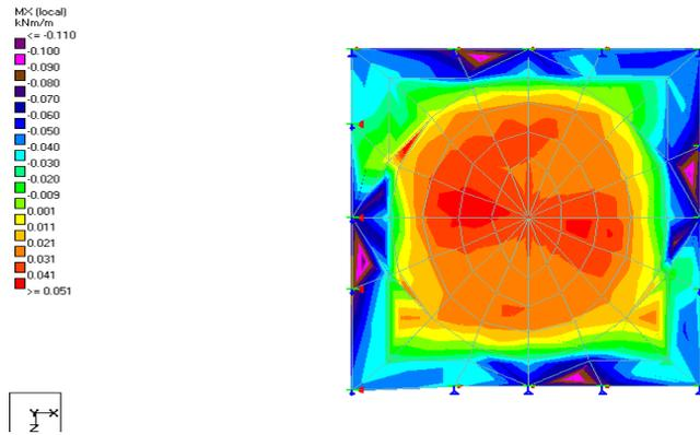
Fig. 5b - Sx Local Stress of Panel 0.5m X 0.625m
