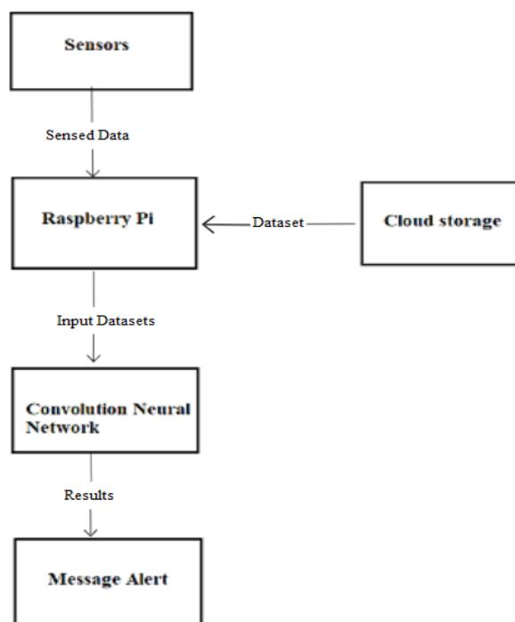
When a vehicle which is installed with this proposed system and entered into field and it can be controlled by a remote and user can have this in his mobile also. Once the pictures of leaves are collected, then they are stored in cloud. Pictures will serve as inputs to the convolution neural network model which is already trained.
