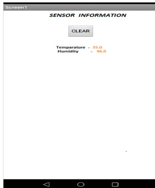
User can view the information collected by sensors instantaneously using mobile application. Moisture threshold level will be given as input and above that threshold motor will on automatically.
