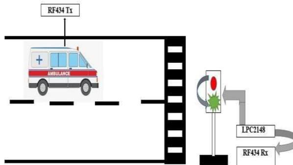
Fig. 5 – Extending the Green Light Time Delay
