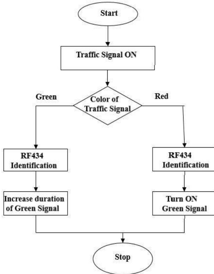
Every emergency vehicle is attached with an RF434 transmitter module (Radio Frequency module). RF434 receiver module is interfaced with LPC2148 is placed at the traffic junction. Essentially, the problem with the emergency vehicle is that it requires its road and path to be cleared so that it can reach its designated location on time and avoid any loss of life or property. The priority can be given by when an emergency vehicle approaches an intersection, the green light can be set too high.
