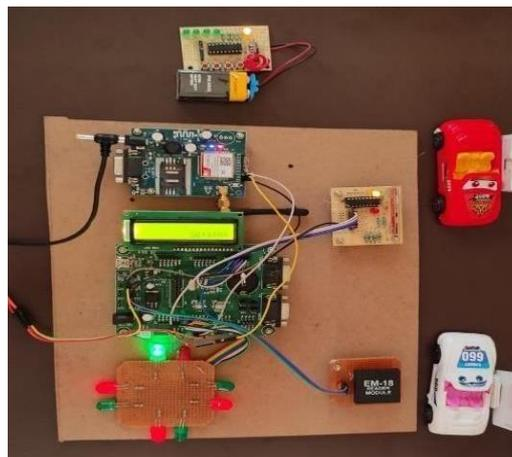
Fig. 11 - RF434 Transmitter Module with Push Buttons Indicating Priority for 4 Directions
