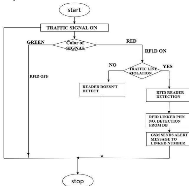
According to Fig. 8, when the signal light is Red if any vehicle jumps the signal, the RFID tag attached to the vehicle is read by the RFID reader. The mobile number which is linked with the unique RFID tag is retrieved and an alert message is sent through the GSM module.
