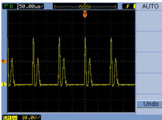
The inductor current ( $I_L$ ) is calculated by using a current probe that is set at 100 mV/A. The average current to be calculated is 0.14 A. The Resonant Inductor current ( $I_{Lr}$ ) was measured according to the same procedure and was 0.5 A (peak-peak).
