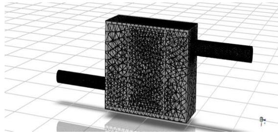
Fig. 5 - Meshed Geometry of Muffler
