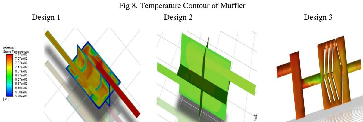
The temperature contour [figure 8] shows the temperature distribution all over the chambers. The temperature distribution varies in all the designs. In design 1 and design 3, the temperature varies from maximum to minimum in all the chambers. In the design 2, the temperature is moderate throughout all the chambers. The temperature varies according to the engine parameters. The value of the minimum temperature is 578K and the maximum temperature is 777K.
