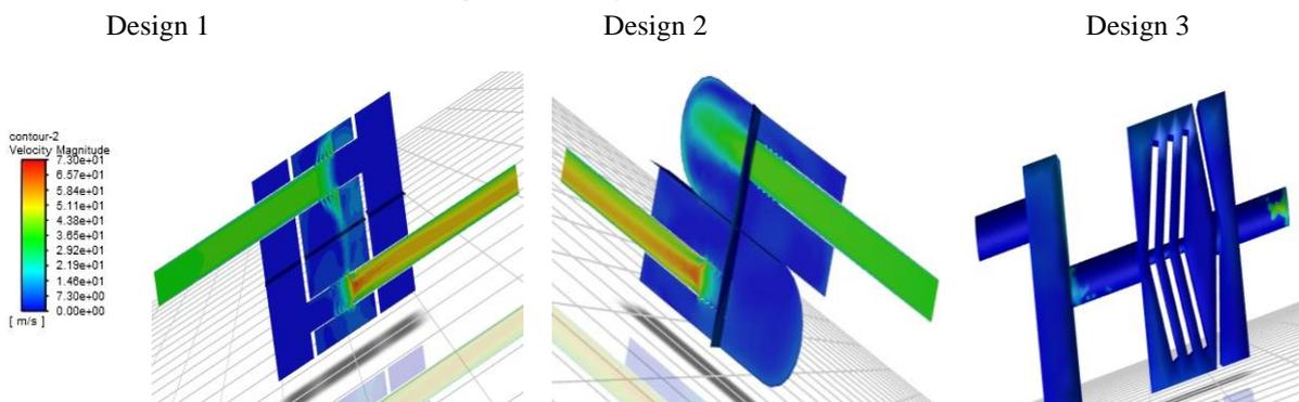
The pressure is inversely proportional to the velocity. The velocity contour [figure 7] shows that the minimum velocity in the inlet pipe and uniformly in other chambers then maximum in the outlet pipe. The maximum velocity value is 73 m/s and the minimum velocity value is 0 m/s. Due to the pressure drop, the velocity at the outlet pipe is much higher. The velocity in the design 1 and design 2 shows that ununiformed flow or the uneven distribution over the chambers. The design 3
