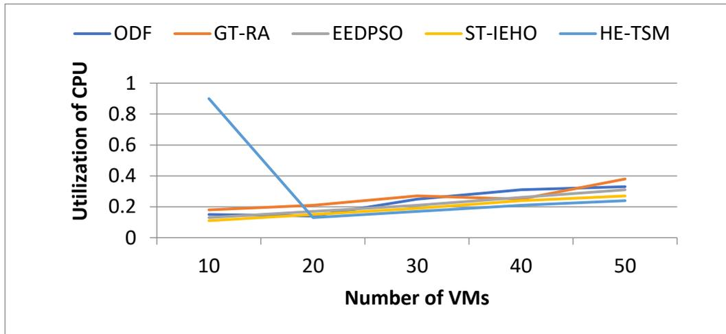
In the figure. 2, the resources utilizations of proposed HE-TSM is better than ST-IEHO, EEDPSO, ODF and GT-RA method. The proposed HE-TSM method provides best CPU utilization. This helps to improve the energy competence of cloud data centre.
