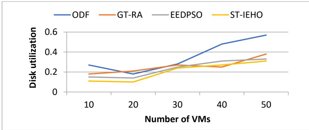
Disk usage was also examined with the four procedures. Outcomes indicated in Figure 4. Thus, the proposed HE-TSM approach has a greater energy competence than ST-IEHO, EEDPSO, ODF and GT-RA that is significant for cloud service provider.
