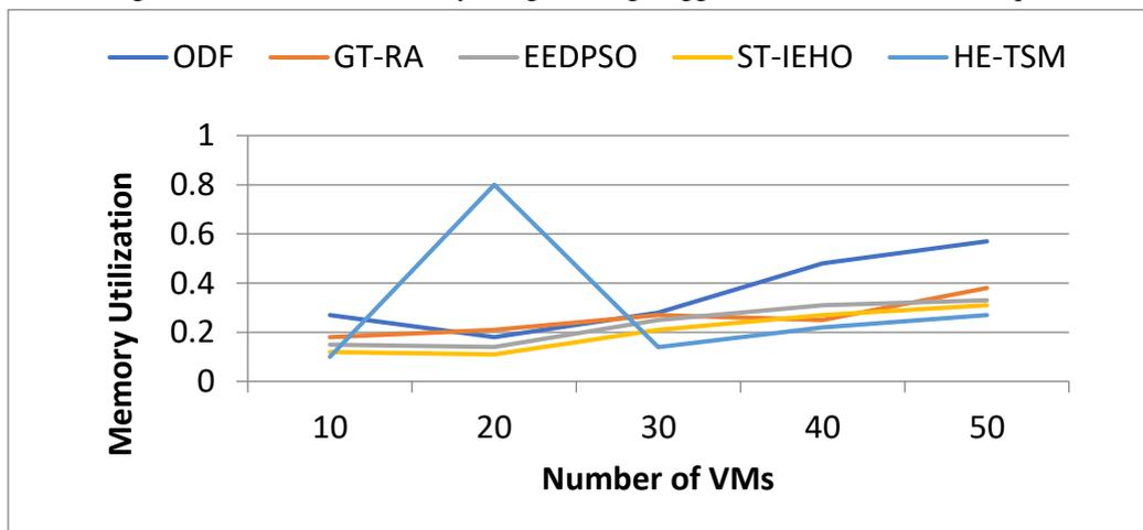
As shown in Figure 3, the memory utilization increases with the increasing order of virtual machines. indicated that the memory usage differs about linearly for conventional heuristic procedures: ST-IEHO, EEDPSO, ODF and GT-RA method. Energy competence of suggested HE-TSM is always greater than ST-IEHO, EEDPSO, ODF and GT-RA with the same number of virtual machines.
