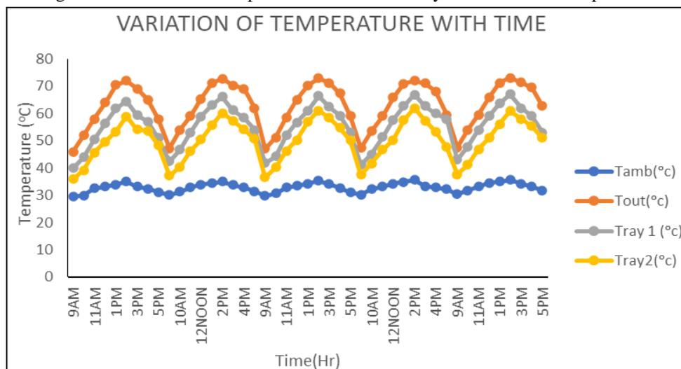
The figure 17 shows that variation of dryer temperature and ambient temperature with time(Hr). The maximum temperature of 72.9°C at Tout and 66.4°C at tray1 and 61°C at tray2. The average temperature at the dryer is 55.5°C as been obtained. During this experiment the maximum temperature of dryer is 72.8°C at the ambient temperature of 35.6°C.
