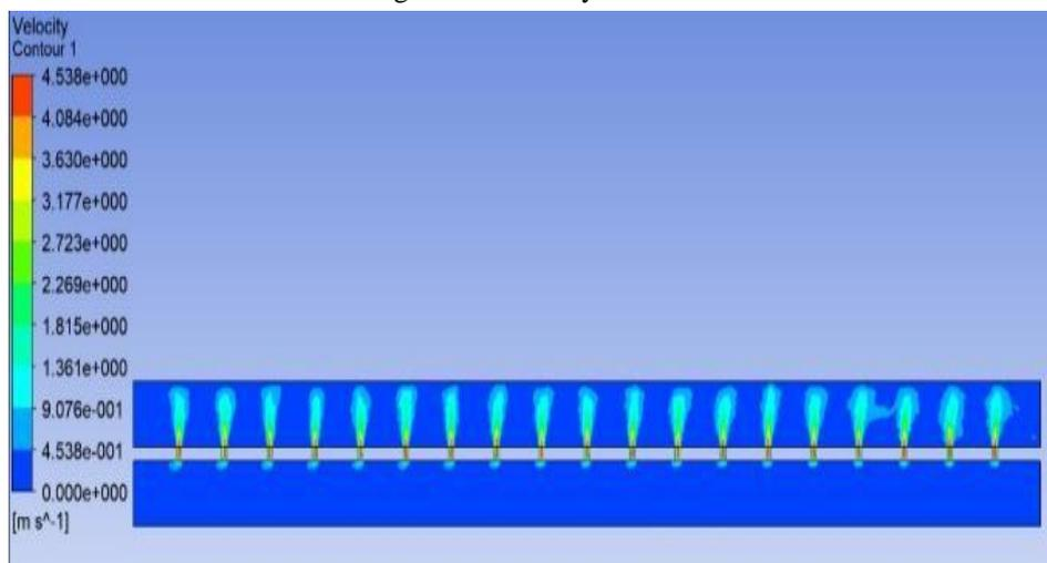
The 3D model has been designed by using Solid Works software. Then it is imported in ANSYS. After importing of the model the meshing has been created by ANSYS ICEM software and therefore meshing created elements consist of around 28 millions elements. The created mesh is imported in ANSYS FLUENT software and the values taken from experimentation are used while simulating collector.
