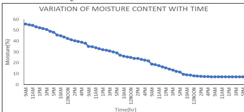
The figure 14 shows that variation of moisture content of copra and time. The average moisture content of copra get reduced from  $55.72\%$  to  $7.08\%$  in 63 hrs.
