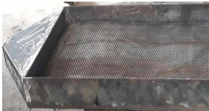
The new fresh copra are used for drying, 6-8mm thickness of copra was selected. The copra are placed uniformly on the two trays. The mass of 2.5kg of copra are used for drying in the chamber. While performing this experiment completely closed the door to prevent from thermal leakages. During this process the solar dryer as been tested under by solar radiation, humidity, moisture level of copra for every one hour interval of time.
