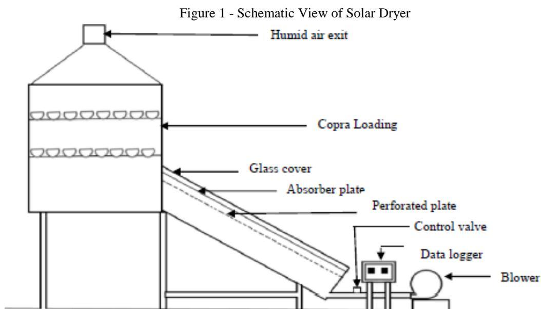
Testing as been done in the month of January, the dryer was fixed under the sun with facing south directions to get better performances. Here we used pt-100 sensor which indicate the maximum accurate range of temperature. Here we using DHT22 Sensor for measuring the humidity of air at higher accuracy. In this experiment we used TES 1333 Solar power meter for measuring the solar intensity with better accuracy. Temperature reading as been recorded on hourly ranges starting from 9AM – 4PM.
