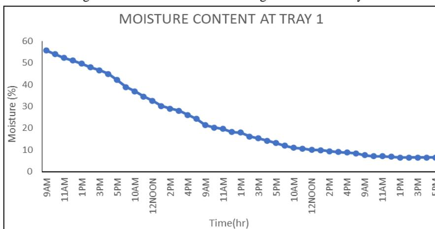
The figure 15 shows that variation of moisture ranges of copra and time. The average moisture content get reduced from the range of 55.64% to 6.5% at 45hours. The moisture reduced from 55.64% to 6.5% in tray 1 at 41hours and tray 2 at 45hours shown in the figure 16.
