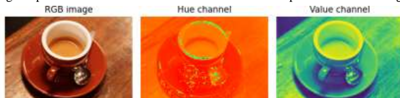
Fig. 5 - The Image Represents the Hue and Value Channel which is Separated from the Original RGB Image
