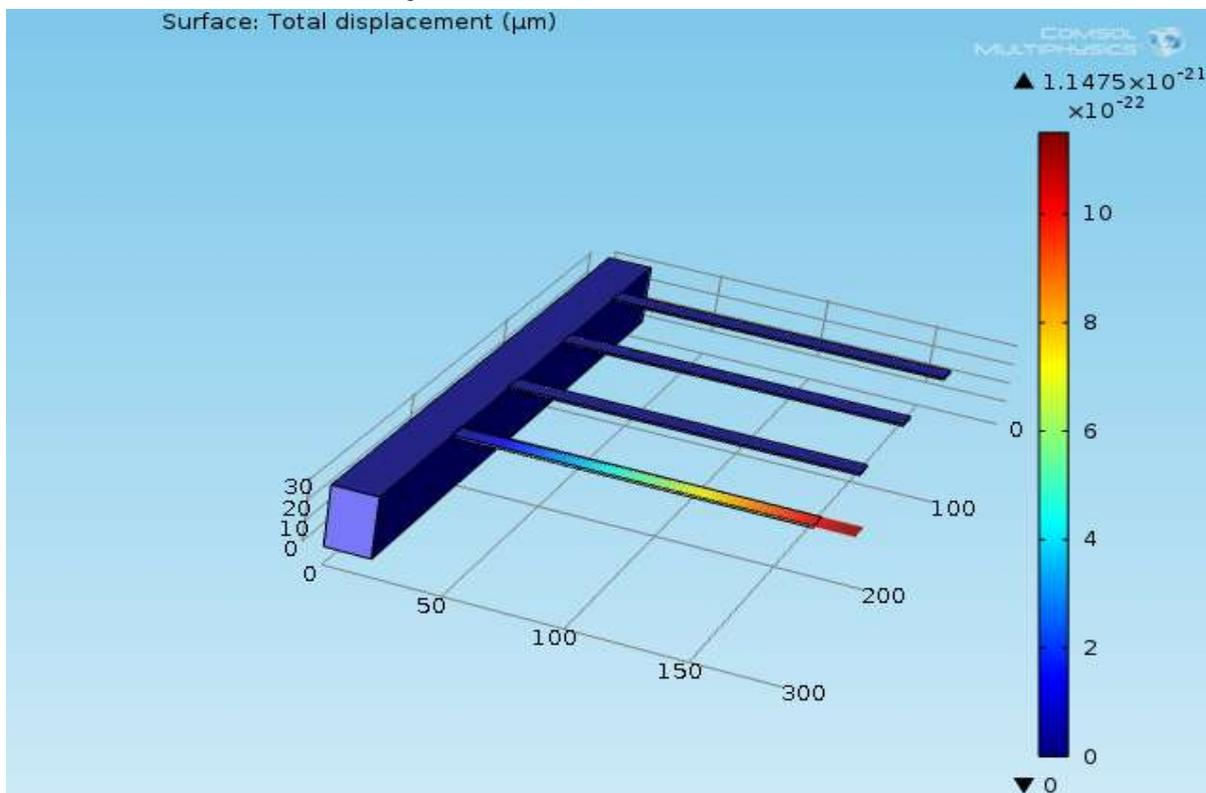
Second beam is taken into account for hepatitis detection applying Si as the material and the corresponding pressure.
