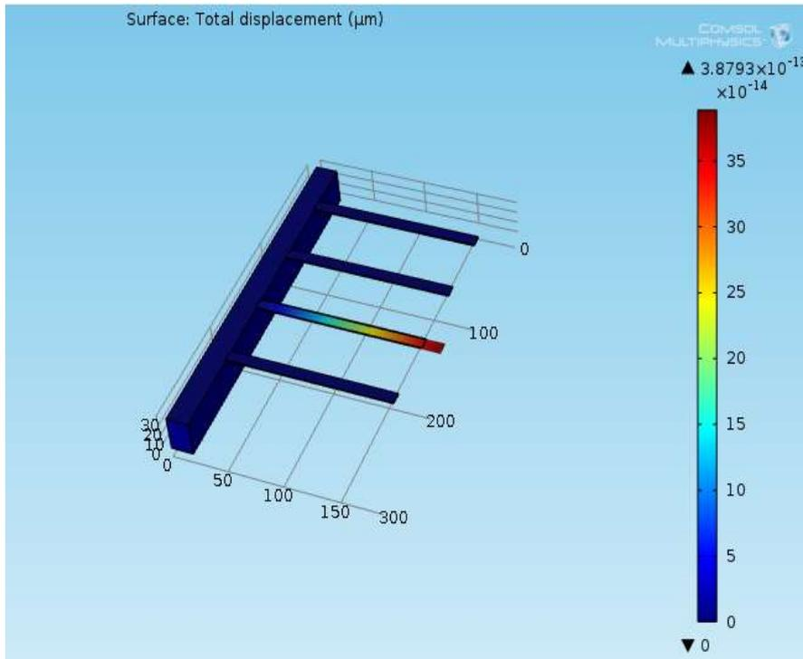
Third beam is taken into account for tuberculosis detection applying gold as the material and the corresponding pressure.
