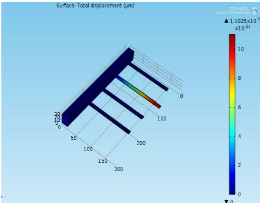
Fourth beam is taken into account for dengue detection applying silicon nitride as the material and the corresponding pressure.
