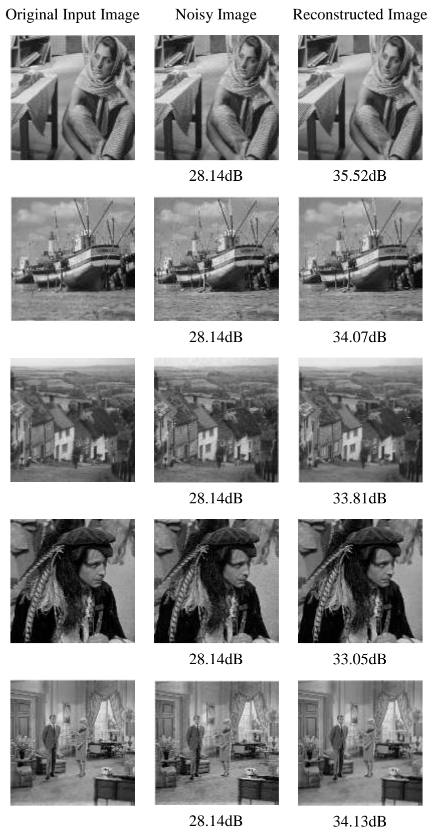
Figure 2- Results of Weighted NNM method with noise standard deviation 10 for input images6 to 10
