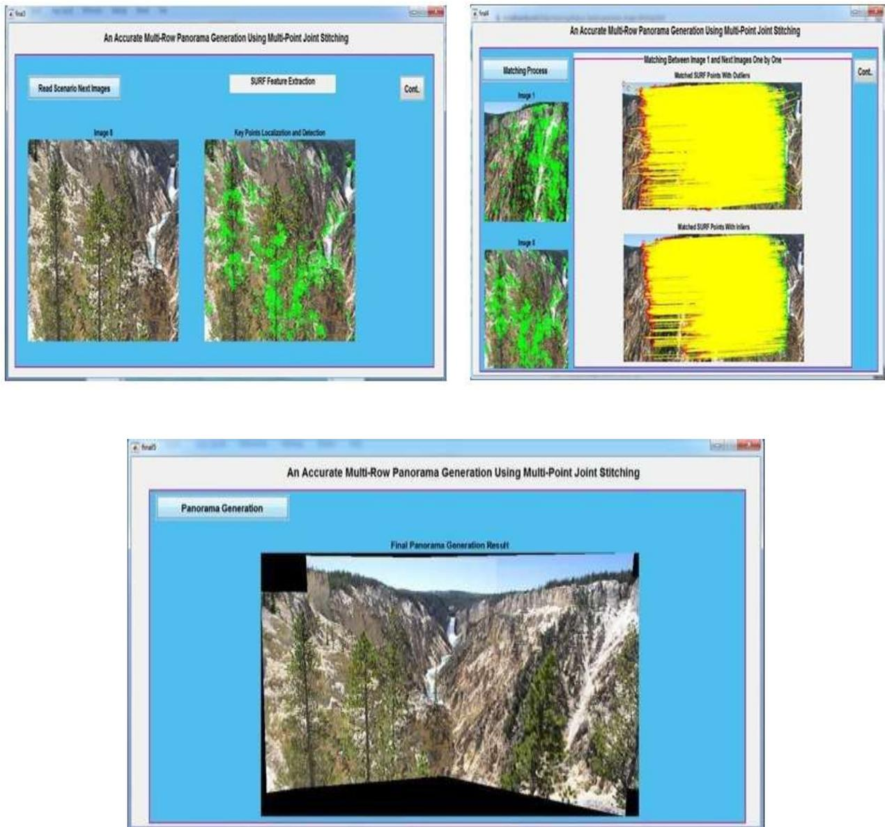
By using the SURF feature based algorithm multiple rows or multiple columns can be stitched at a time so that more accurate multirow panorama can be generated.
