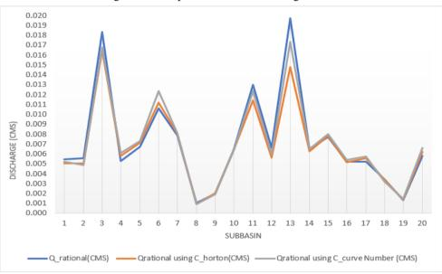
Figure 8 - Comparison of Peak Discharge Values
