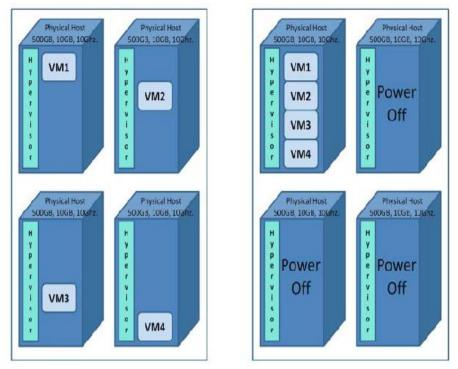
Fig. 3 - Data Center without Server Consolidation; Fig. 4 - Data Center after Server Consolidation
