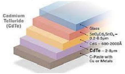
Figure 6 - Cadmium Telluride Solar Cell [11]
