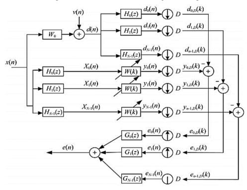
Figure 3.2 - Structure of the Subband Adaptive Filtering
