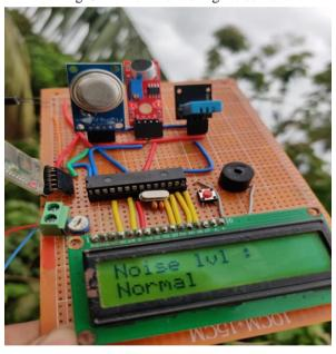
As we can see in fig. 10 and 11 the device is monitoring and detecting the vales for air composition and it is detecting for noise level in the atmosphere after detecting the device will display the amount of carbon mono oxide, toluene, ammonia, alcohol, carbon dioxide and acetone. The device also displays the noise composition in the atmosphere and detects if there is presence of fire.
