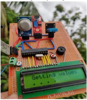
Fig. 3.10 - IoT Monitoring Air Composition
