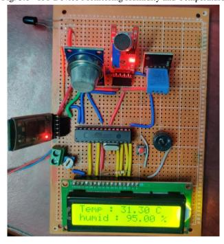
Fig. 3.8 - IoT Device Monitoring Humidity and Temperature
