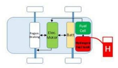
Internal Structure of Fuel Cell E-Vehicle
