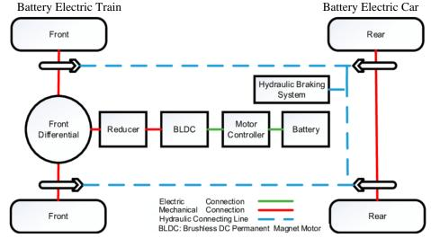
Internal Structure Battery E - Vehicle
