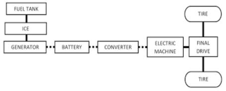
Internal Structure of Range Extened E-vehicle
