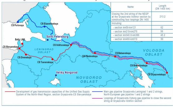
Fig. 2 - Formation of the Gas Transmission System of the Nord Stream 2 Project
