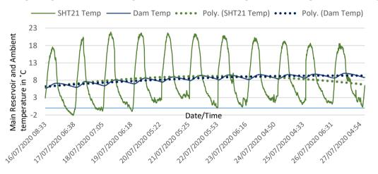
Figure 2. Graphic representation of atmospheric and main reservoir temperatures for the period 16 - 27 July 2020
