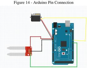
Arduino pins are connected and simulated. The waste is fed through conveyer belt and direction is controlled by motor and the motor drive. On metal detection message is displayed on the monitor, who says it's a metal waste, and then the waste is chucked out, and remaining waste is sent through the IR sensor, where plastic waste is rejected and the motion of conveyer belt is controlled by
