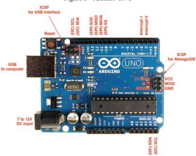
IOREF: This stick on the Arduino/Genuino board provides the voltage reference using which the microcontroller works. The IOREF pin voltage picks the fitting force source on the yields with 5V or 3.3V.
