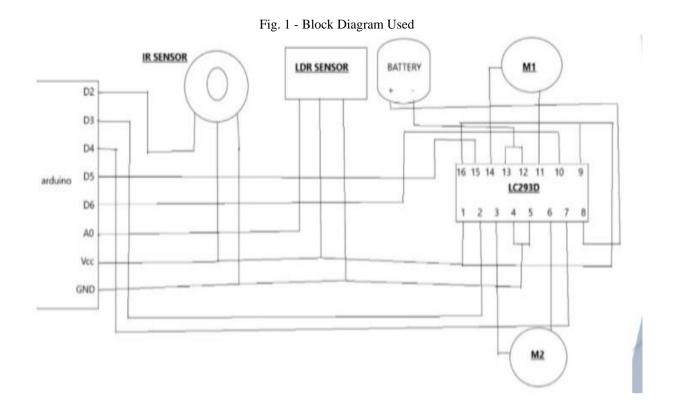
The circuit we map out here is H-Bridge circuit. This circuit is used to run two motor at a time.
