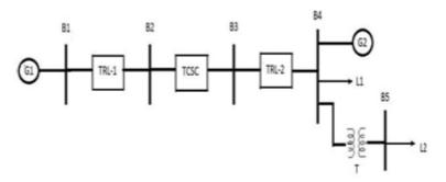
Fig:1.Flow diagram of the proposed test system.
