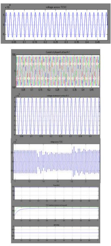
**Map: 3.** TCSC in Good Condition: (I) phase – A voltage at Bus bar B - 2, (II) phase – A current at Bus bar B – 2, (III) TCSC potential difference, (IV)TCSC power flow, (V) TCSC impedance and (VI) TCSC angle.
