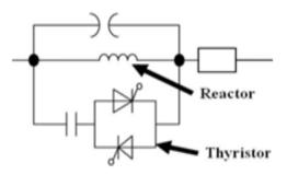
Fig:2. Schematic figure of the TCSC
