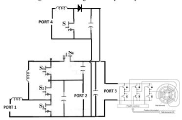
Fig. 3 - Circuit Diagram of Proposed System
