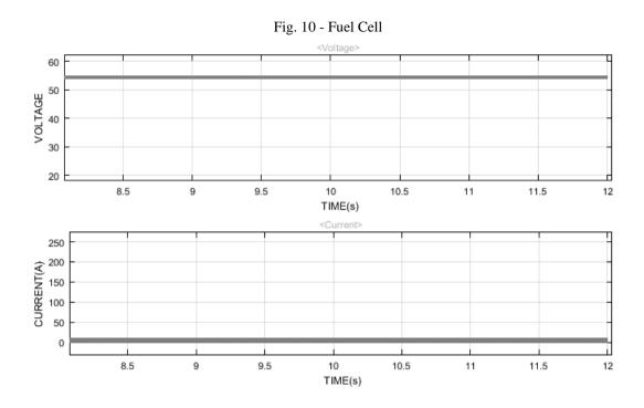
Fuel cell has constant voltage supply, irrespective of any changes. When the output voltage (V out) is high, current (I) is low.
