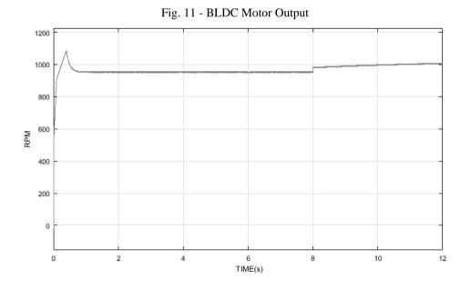
This graph shows the final output of our system, that is how to motor runs with various inputs. The rotation per minute is 1000 rpm which is achievable. Thus, it also replicates the normal electric vehicles' output.
