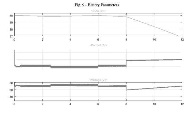
State of charge is associated with battery tells how much power can it deliver in ampere hours (Ah). At a particular time when battery loses its energy the voltage drops and current raises. In this situation, the bidirectional port is used to recharge the battery. Simultaneously, other source comes in.
