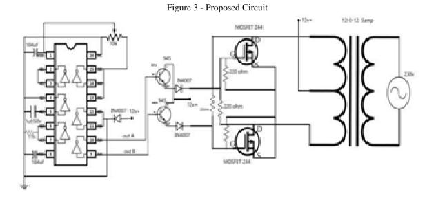
This is the propose circuit for inverter section. Here multivibrator CD4047 is used. This is the astable multivibrator. The output of the astable multivibrator is square wave since AC circuits works on pure sine wave so the square wave signal is sent to two MOSFETs IRZ44 which trims into pure sine wave and connecting to transformer. From transformer, connection is connected to the load.
