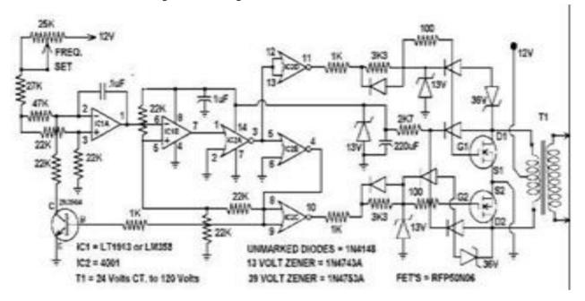
Figure 1 - Existing Circuit for 20 Watts Power Production
