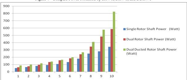
Figure 4 - Compare Power Produced by SRWT, DRWT, and DDRWT
