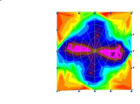
Fig. 5c - Sqx Local Stress of Panel 0.5m X 0.625m
