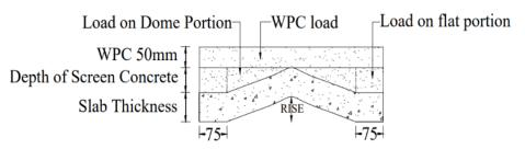
Fig. 2 - Panel and Floor Finishes Thickness
