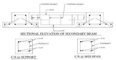
Fig. 7 - Reinforcement Details of Secondary Beam Resting on Primary Beam
