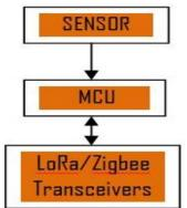
We designed and programmed our proposed energy model algorithm for sensor node A and B, such a way that measured sensor data transmitting to sink node A and B in cyclic sleep modes.
