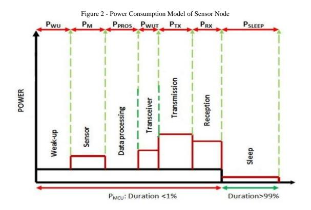
The working of sensor node is characterized by variable time durations. Figure 2 illustrates achievable working time duration of the sensor node in different operating modes, which are maneuver by the Central processing Unit. In this proposed model, power consumed by the sensor node A and B for one cycle is given by equation 1.
