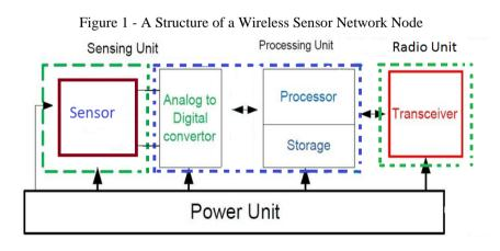
Sensing, processing, power source and transceiver unit are four major modules in wireless sensor node architecture. *Sensing unit:* Sensors and module are the electronic devices that detects and respond to some type of input from the physical environmental conditions, these parameters are in analog form and converted in to digital format. *Processing unit:* acquisition of an output signal from the sensor unit, process the data after accession and communicate data to the transceiver. *Power*
