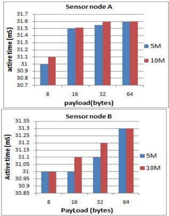
Figure 11 - Payload vs. Mean Active Times (ms)
