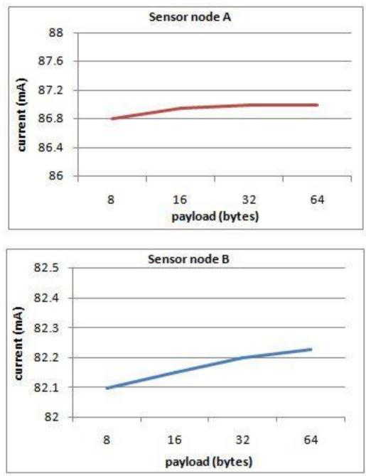
Figure 12 - Active Current Consumption vs. Payload
