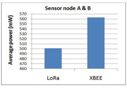
Figure 13 - Average Power Consumption of Sensor Node A & B
