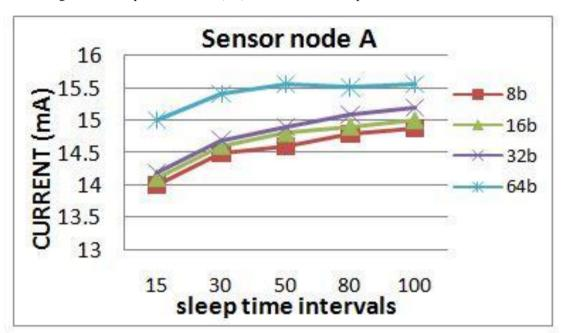
Figure 10 - Sleep Time Interval (sec) vs. Current Consumption of Sensor Node A and B
