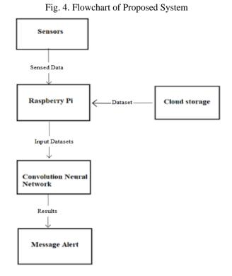
When a vehicle which is installed with this proposed system and entered into field and it can be controlled by a remote and user can have this in his mobile also. Once the pictures of leaves are collected, then they are stored in cloud. Pictures will serve as inputs to the convolution neural network model which is already trained.
