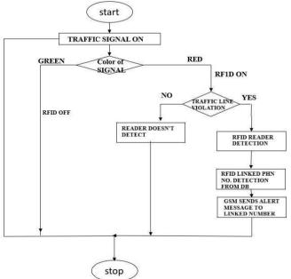
According to Fig. 8, when the signal light is Red if any vehicle jumps the signal, the RFID tag attached to the vehicle is read by the RFID reader. The mobile number which is linked with the unique RFID tag is retrieved and an alert message is sent through the GSM module.
