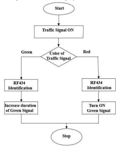
Fig. 6 - Flow Chart of the Emergency Vehicle Clearance
