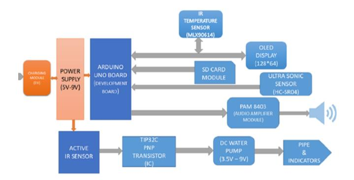
The Contactless Sanitization and Temperature Monitoring System is responsible for analyzing temperature and produces audio output. After completing the temperature test further we proceed with a sanitizer to hygienic our hands.
