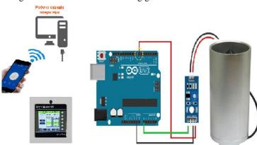
Figure 2 - A device for monitoring grain moisture in real time
