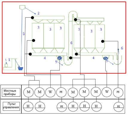
1-grain washing; 2-distribution auger; 3-capacitive hopper; 4-mixer auger; 5-humidity control device; 6-screw mixer;
