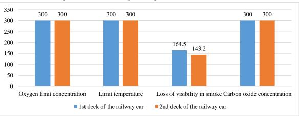
Figure 9. Time of blocking the escape routes in the double-deck car
