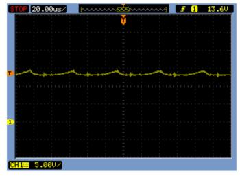
Fig. 7(c) - Filter Capacitor voltage (V<sub>c</sub>) of Buck ZVS MRC
