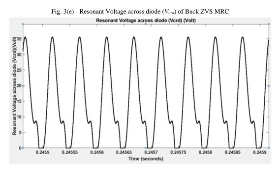
From Fig. 3(a), the average value of the inductor present is 0.15 A. The peak-peak value of the resonant inductor current present in Fig. 3(b) is 0.5 A and the frequency is 20 kHz. The average output voltage of Fig. 3(c) is 14 V. The peak resonant voltage across switch of Fig. 3(d) is 35 V with a frequency of 20 kHz. The peak resonant voltage across diode of Fig. 3(e) is 35 V with a frequency of 20 kHz. All these values logically obey equations.
