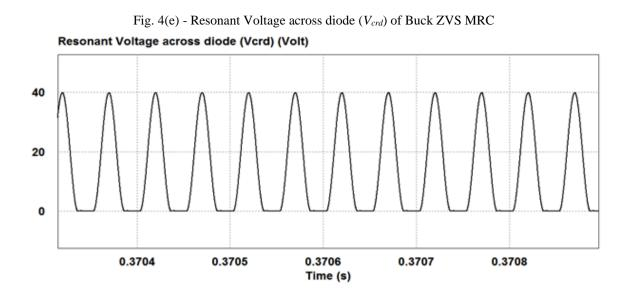
Fig. 4(a) reveal that the average inductor current value is 0.16 A. The maximum-maximum value of the resonant inductor current from Fig. 4(b) is 0.52 A and the frequency is 20 kHz. The average output voltage of Fig. 4(c) is 13 V. From Fig. 4(d), the peak resonant capacitor voltage across switch is 40 V, and the frequency is 20 kHz. From Fig. 4(e), the peak resonant capacitor voltage across diode is 40 V, and the frequency is 20 kHz. Both these values technically obey the equations.
