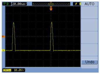
Fig. 7(e) - Resonant Voltage across diode (V<sub>crd</sub>) of Buck ZVS MRC
