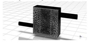
Fig. 4 - Meshed geometry of Muffler
