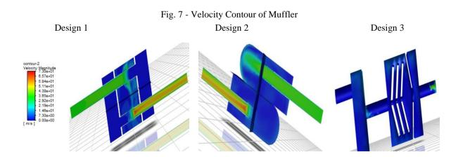
The pressure is inversely proportional to the velocity. The velocity contour [figure 7] shows that the minimum velocity in the inlet pipe and uniformly in other chambers then maximum in the outlet pipe. The maximum velocity value is 73 m/s and the minimum velocity value is 0 m/s. Due to the pressure drop, the velocity at the outlet pipe is much higher. The velocity in the design 1 and design 2 shows that ununiformed flow or the uneven distribution over the chambers. The design 3
