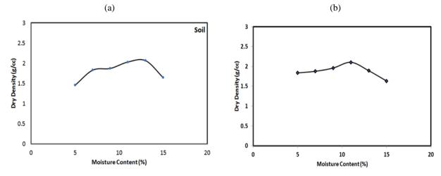
Table 3 - Comparison of OMC and MDD (Mean and Standard error of mean) for soils with and without marble dust. TheOMC decreases by 13% and MDD increases by 1.8% when 5% marble dust is added.
