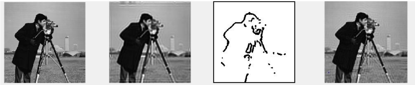
Fig. 1 - Simulation results of image deblurring and it corresponds to a relatively small network. It is composed of four layers that the original image can appear in Fig.1a, Deblurring with INITPSF can appear in Fig.1b and weight array can appear in Fig.1c and at last the deblurred image can appear in Fig.1d.
