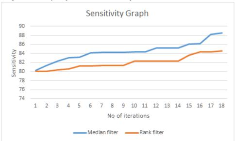
Fig. 9 - Sensitivity Graph which shows the comparison of median filter and rank filter
