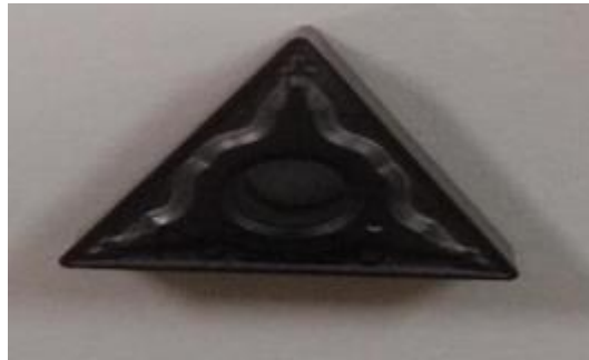
Fig. 2 - Uncoated insert - Specification- TNMG 160408 EN - CF; CF - Negative relief angle; Insert included angle 60 degrees, Cutting edge length 16.5 mm; Insert thickness 4.76 mm; Corner radius 0.8 mm; Cutting edge condition code E - Rounded; Insert hand N-Neutral; Fixing hole diameter -3.81 mm
