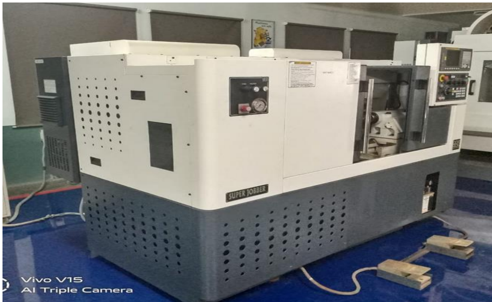
Fig. 3 - CNC Machining centre - Super jobber - Specification: Swing over bed -500 mm, Swing over carriage - 260mm, Maximum turning dia - 320 mm, Maximum turning length - 400 mm, Distance between centres - 425 mm, Maximum spindle speed - 3500 rpm, No. of stations - 8)
