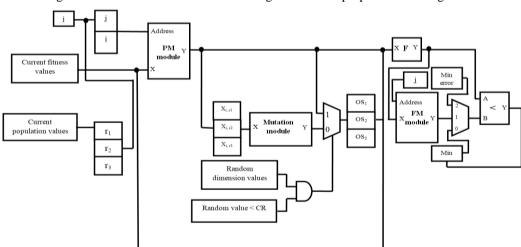
Figure 3- The entire scale hardware arrangement in the proposed CWO algorithm
