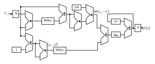
Figure 6 - Blocks of Fitness Function Module based on Rosenbrock's Function
