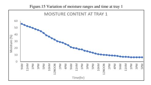
ISSN: 2237-0722 Vol. 11 No. 4 (2021) Received: 07.01.2021 – Accepted: 28.05.2021 The figure 15 shows that variation of moisture ranges of copra and time. The average moisture content get reduced from the range of 55.64% to 6.5% at 45hours. The moisture reduced from 55.64% to 6.5% in tray 1 at 41hours and tray 2 at 45hours shown in the figure 16.
