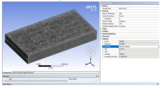
Figure 4 - Mesh Generation in CFD
