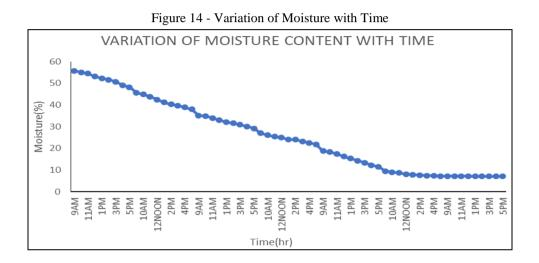
The figure 14 shows that variation of moisture content of copra and time. The average moisture content of copra get reduced from 55.72% to 7.08% in 63 hrs.
