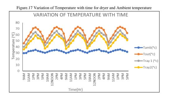
The figure 17 shows that variation of dryer temperature and ambient temperature with time(Hr). The maximum temperature of 72.9°C at Tout and 66.4°C at tray1 and 61°C at tray2. The average temperature at the dryer is 55.5°C as been obtained. During this experiment the maximum temperature of dryer is 72.8°C at the ambient temperature of 35.6°C.
