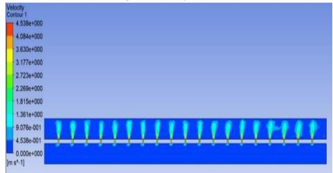
The 3D model has been designed by using Solid Works software. Then it is imported in ANSYS. After importing of the model the meshing has been created by ANSYS ICEM software and therefore meshing created elements consist of around 28 millions elements. The created mesh is imported in ANSYS FLUENT software and the values taken from experimentation are used while simulating collector.
