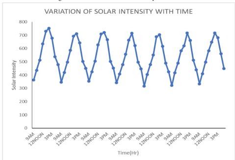
Figure 12 - Variation of Solar Intensity with Time
