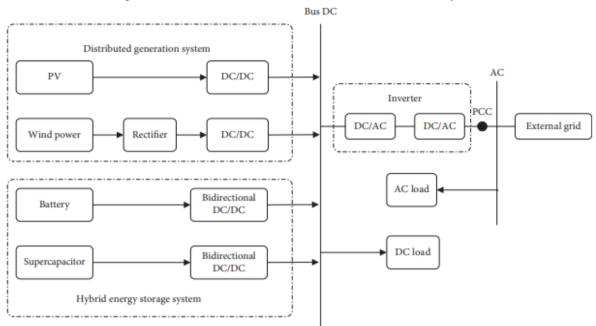
Figure 2 - Illustration of the Grid-connected HES Generation System
